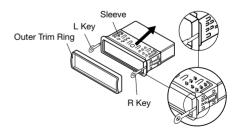
5. Mount the sleeve by inserting the sleeve into the opening of the dashboard and bend open the tabs located around the sleeve with a screwdriver. Not all tabs will be able to make contact, so examine which ones will be most effective. Bending open the appropriate tabs behind the dashboard to secure the sleeve in place.
